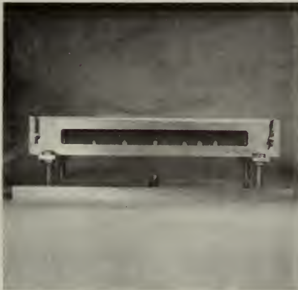
Figure 9 - Film holder. Left: Front view. Note height adjustment screws and lead markers. Right: Plan view. Note curvature of holder and approximate energy scale.
